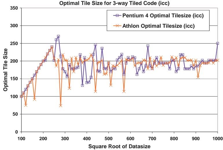
Fig. 8. Optimal tile size on Athlon and Pentium 4-M processors, for each data point from Figure 7. These results are based on a straight-forward exhaustive search implemented using the TaskGraph library’s runtime code restructuring capabilities (see code in Figure 6).
