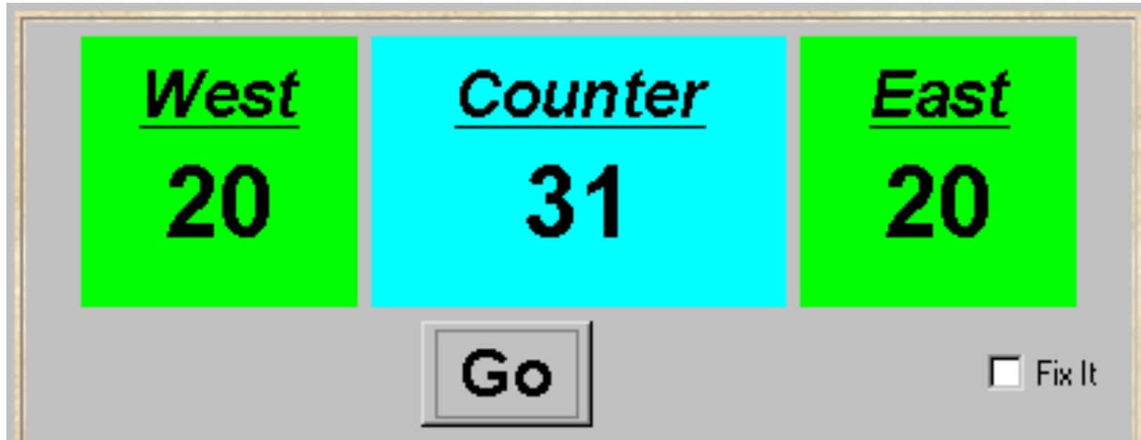
After the East and West turnstile threads have each incremented its counter 20 times, the garden people counter is not the sum of the counts displayed. Counter increments have been lost.
