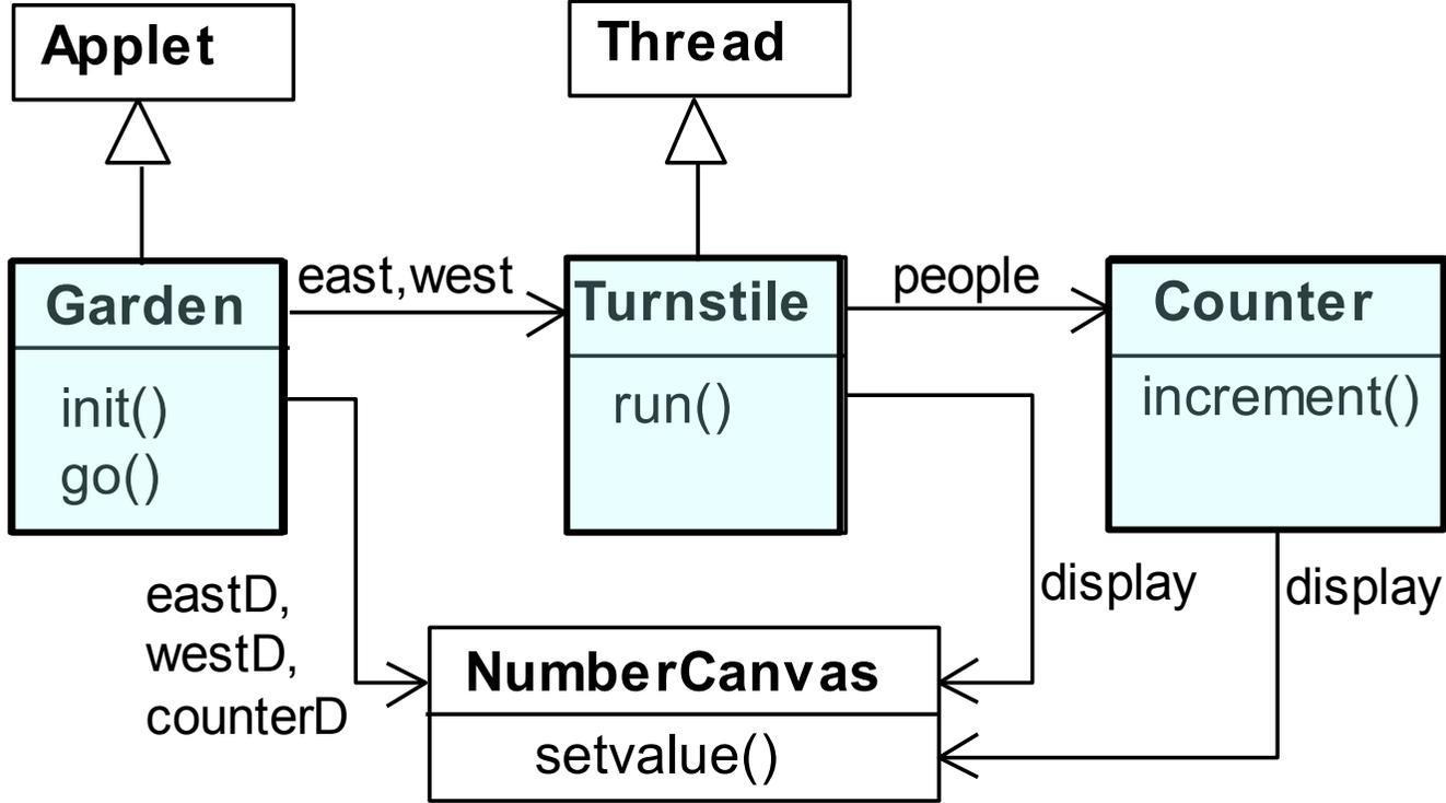
The **Turnstile** thread simulates the periodic arrival of a visitor to the garden every second by sleeping for a second and then invoking the **increment()** method of the counter object.
