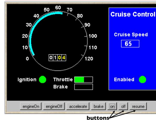
When the car ignition is switched on and the **on** button is pressed, the current speed is recorded and the system is enabled: *it maintains the speed of the car at the recorded setting.*
