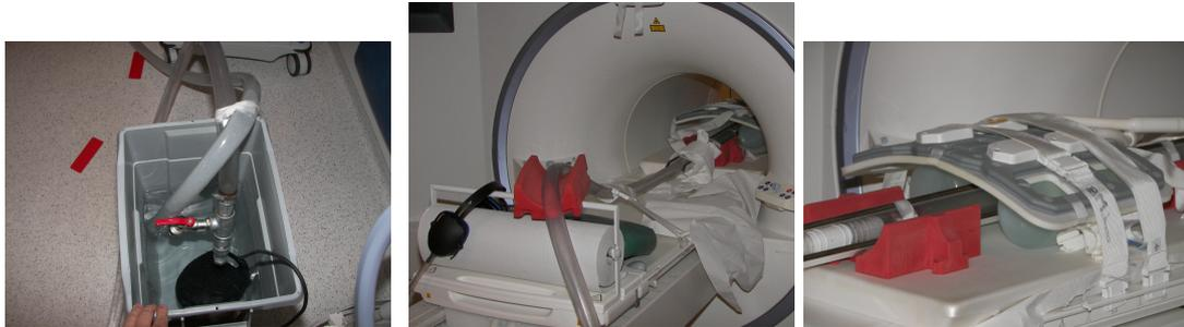
(a) The flow is emulated with a submersible pump and controlled by a valve. The end of the tube closes the circuit in the same tub. (b) The narrowing is placed for the measurements in the iso-center of the magnetic field. (c) Two bottles filled with water enable for the body-coil an equal distance to the tube.
