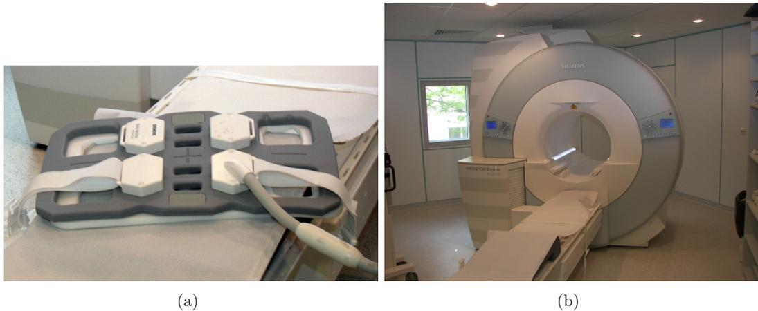
Figure 3.11: A typical body coil for thorax parallel image acquisition (a). This array-coil fits to the Siemens Magnetom Espree Tim [76 x 18] system, situated at Diagnostikzentrum Graz (b).
