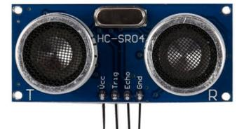
Figure 3: HC-SR04 sensor package
