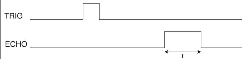
Figure 2: Control signals from HC-SR04 sensor package
