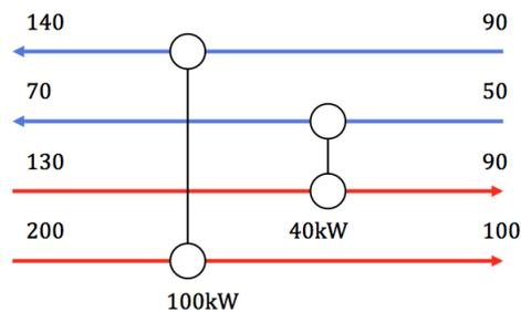
Figure 2.8: An example of how a heat exchanger network with two heat exchangers may look
