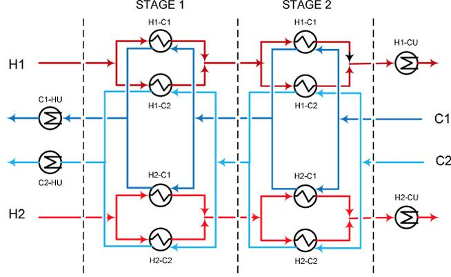
Figure B.1: Two-stage Superstructure for two hot and two cold streams.
